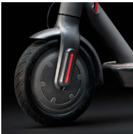
8.5" tyres with air chamber
